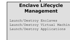
The resources managed by Leviathan can be space partitioned into multiple enclaves. Each enclave runs its own OS/R stack, for example a native Kitten lightweight kernel instance or Linux virtual machine. The Leviathan shell provides commands for forming enclaves, loading virtual machines, and launching applications.
