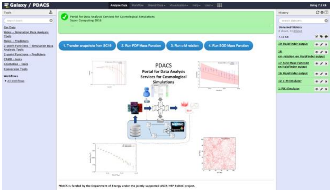
Figure 4: Snapshot of PDACS, a web-based portal that provides a range of analysis tools (shown in the left bar) allowing easy data access and analysis. The user can create complicated workflows by choosing and combining a range of analysis tools that are then run on a back-end cluster. At SC16, PDACS was part of the live demonstration showing how data could be easily pulled from the show floor and analyzed at different facilities. A major advantage for PDACS users is that they do not have to know any details about the cluster where the analysis is carried out (e.g., submission systems, compilers). PDACS handles all these automatically.
